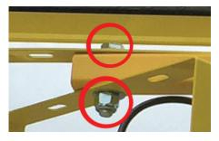
Make sure all power is off. Remove the light fixture wiring from the junction box that sits at the cross bar. Take your existing light fixtures physically off of your light tower right where the yoke meets the crossbar.
